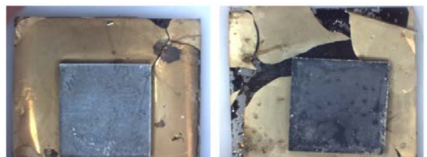
圖9. Glass/SiC/Al/...結構在熱壓合後薄膜剝離
